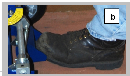
Engage the brakes by pressing down on the brake actuator
