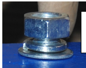
g. Fasten the bolts in place using a flat washer, followed by a lock washer and then a nut.
