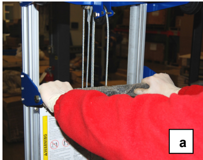
a. Grasp the operator handle at each end. This will provide the greatest degree of steering control.
