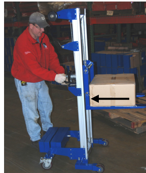
Set the load on the forks. The load must rest against the back of the forks.
